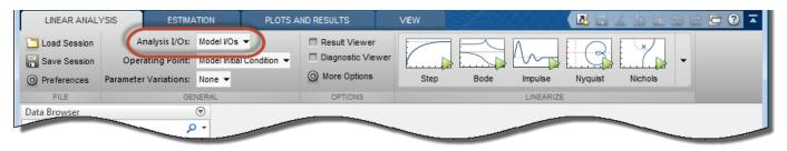
To linearize the model using the specified analysis points and generate a Bode plot of the linearized
